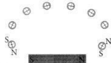
Drawing a magnetic field line with the help of a compass needle
